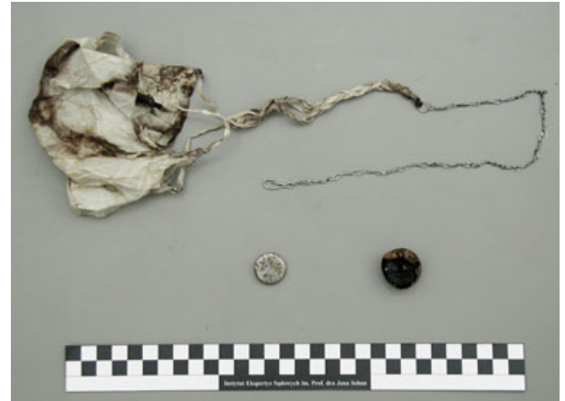
FIG. 3—Parts of a rocket parachute flare found at the dead end of wound channel in the victim's leg.
